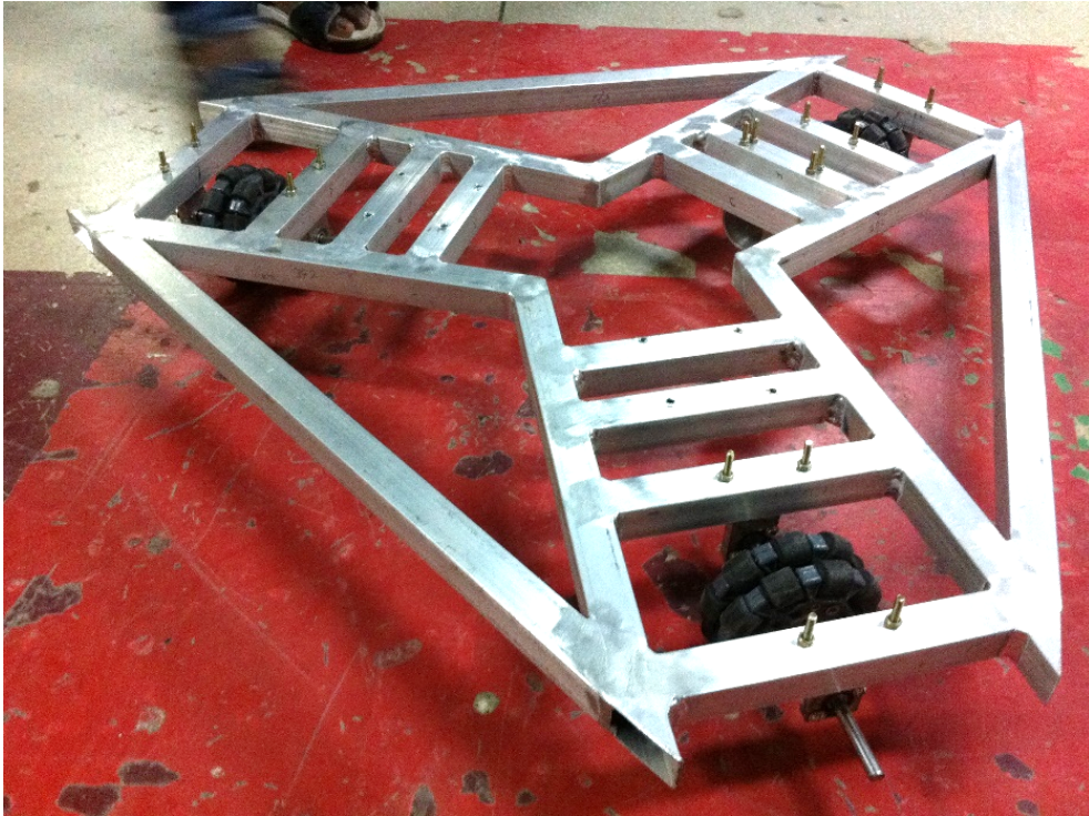
Figure 3.3: Drive base after welding
