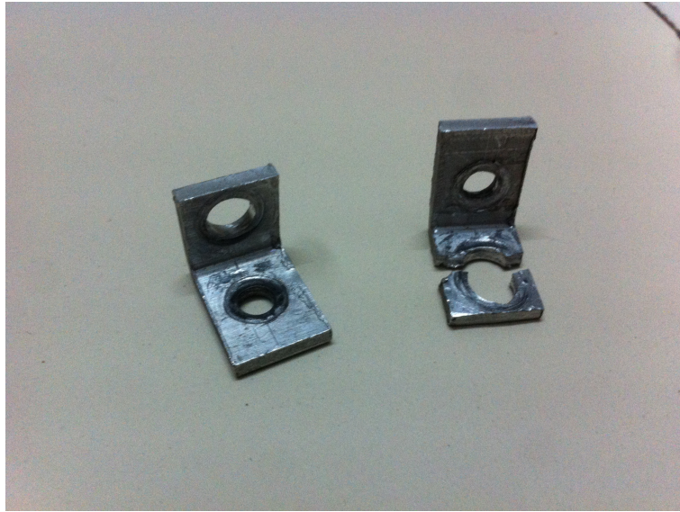
Figure 4.9: A broken L along with another unbroken one, both made of aluminum
