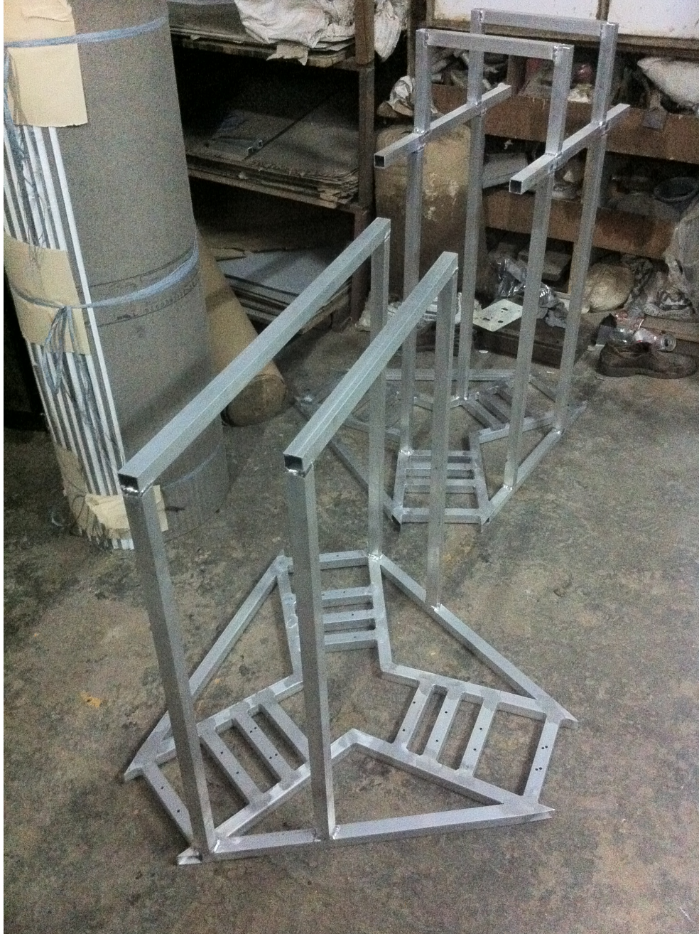
Figure 3.13: The skeletal chassis of the robots after welding
